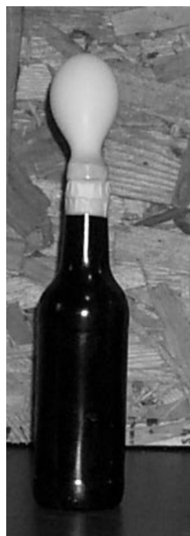
Figure 1: A simple apparatus made of a bottle, balloon and tape used to capture carbon dioxide for quantification during the guided inquiry. Photo by Brian Guercio.
